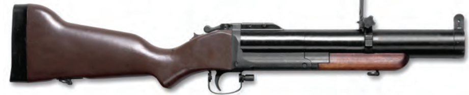
The M-79 had a large flip-up sight midway down the barrel, as well as a leaf foresight at the end of the barrel.
