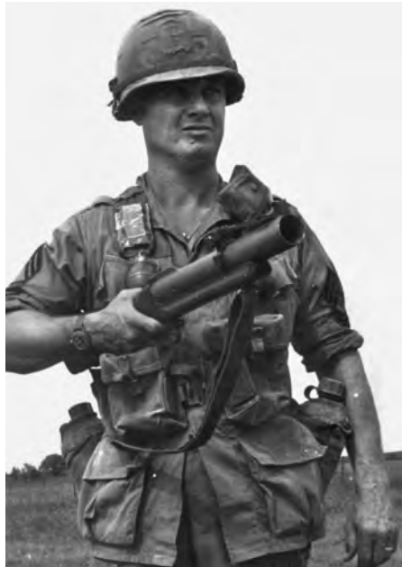
ABOVE: The M-79 was popular with U.S. soldiers serving in Vietnam who found it easy to use, highly reliable, and requiring little maintenance. BELOW: The break-open rear breech made the weapon somewhat slow to load, but that was offset by its 375-meter range and five-yard fragmentation zone.
